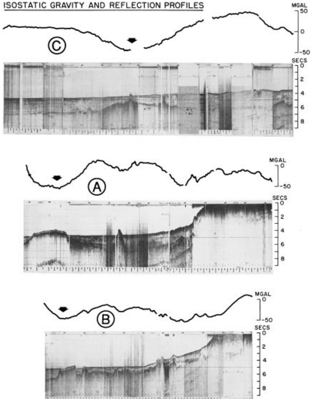
Figure 4. Single channel reflection profiles and 2D isostatic gravity anomalies over Laxmi Ridge (see arrow) from Naini and Talwani (1982).
